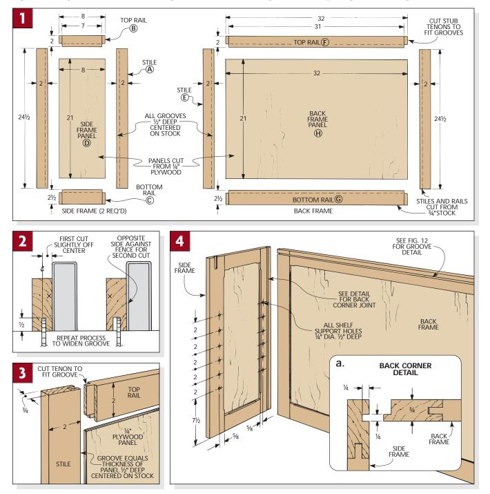
These stub tenons are cut by making multiple passes over the saw blade to leave a tongue that fits the groove.
