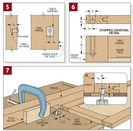
clamp a stop block to the left of the bit on the router table; see Fig. 7. For the right frame, move the stop block to the right of the bit and repeat the cut from the opposite direction.
